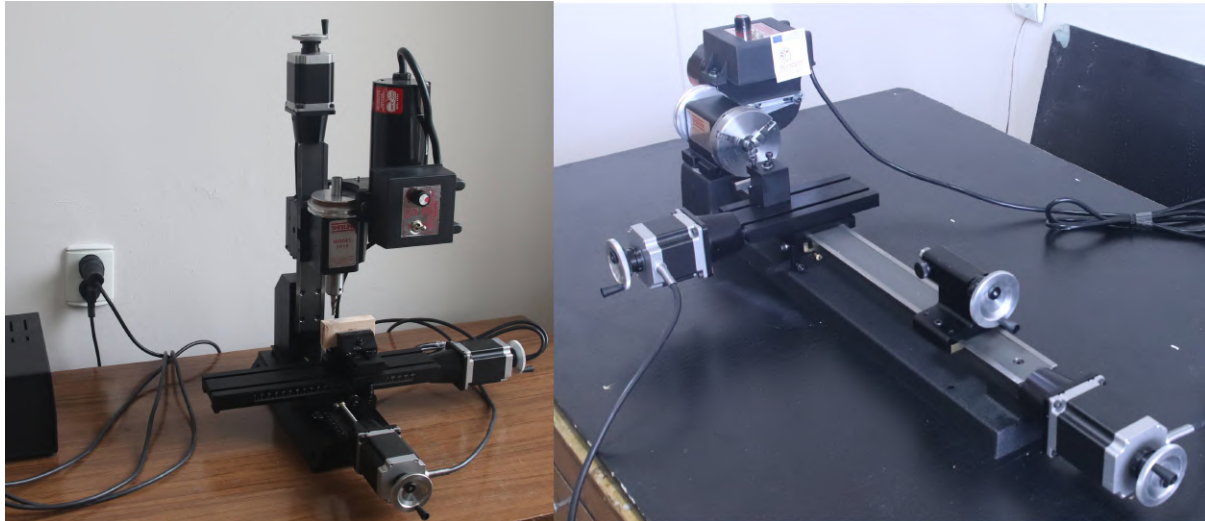
Figure 2: CNC machines: Sherline 5410 CNC and Sherline 4410 CNC.
