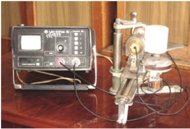
Fig. 4. Stand for measuring the velocity of elongated and transverse waves propagation
