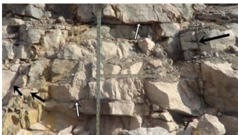
Fig. 2. Fragment of the working face of the granite quarry “Sivach”: the light arrows – compression joints S ; dark arrows – horizontal formation joints L
