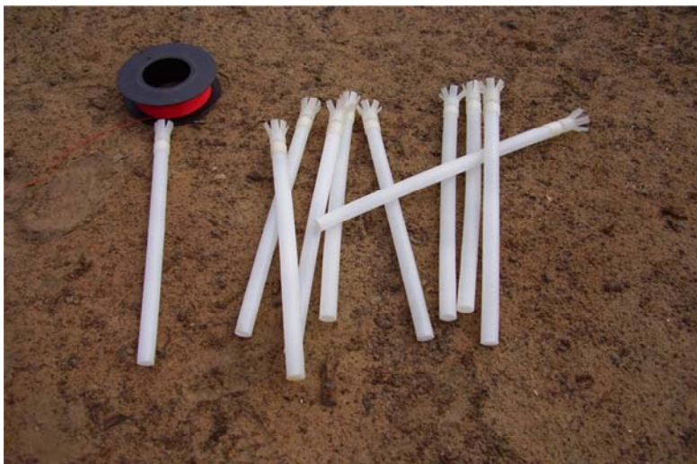
Fig. 1. Domestic elongated charges of the type like K-tubes for splitting of a block stone
