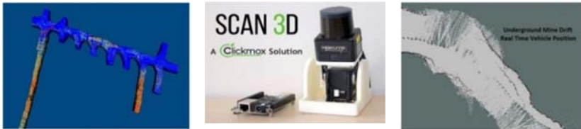
(a) (b) (c) Fig. 17. (a) 3D map of a gallery realized by a 3D Clickmox Scanner; (b) 3D Scanners Systems; (c) Real-time positioning of cars in car galleries using 3D scanners;
