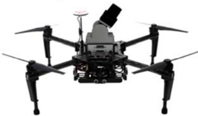
Fig. 16. The DRON MineFly with cartography and 3D scanning ability
