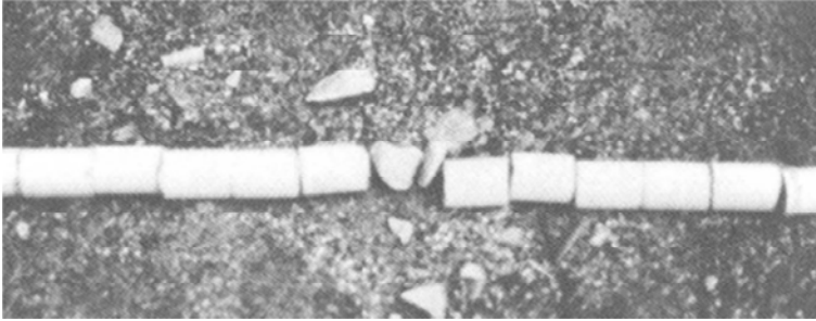
Fig. 2. Disking due to stretching of the cores with a diameter of 5.7 cm from the block 10x10x5,7 m
