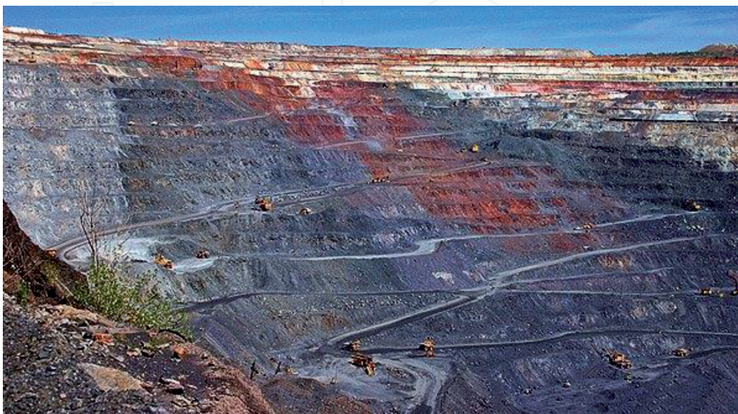
Figure 4. One of the world largest open pits of Ingulets MPP: Depth 520 m, designed capacity by crude ore - 38 Mt./year.
