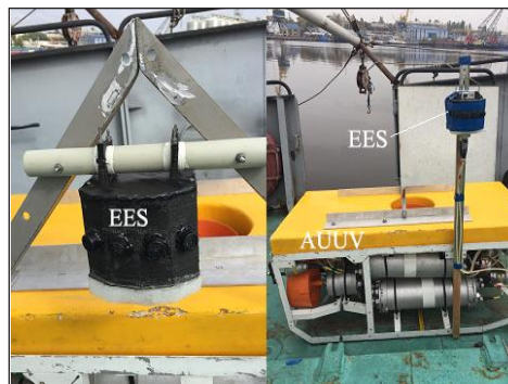
Fig. 6. Exterior of the EES system and its arrangement on the AUUV-1
