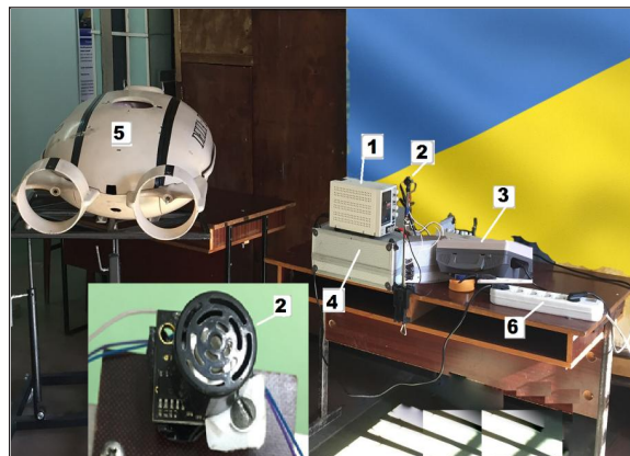
Fig. 2. Exterior of the setup for the construction of the direction pattern of ultrasonic range finders: 1 — power supply; 2 — ultrasonic range finder; 3 — oscilloscope; 4 — auxiliary equipment; 5 — AUUV mockup; 6 — extension cord
