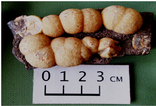
Fig. 3. Spherulitic aggregates of calcite from a void in martitized cummingtonite-magnetite quartzites from an underground working of G.K.Ordzhonikidze Mine.
