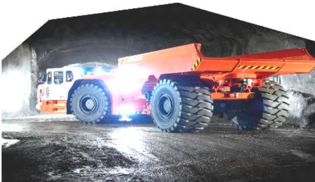
Рис. 3.1. Самоскид SANDVIK TH551i (Джерело: https://www.memoireonline.com/06/24/14603/m_Calcul-de-la-productivite-dun-engin-de-transport-dans-la-mine-souterraine-Cas-de-la-benne-Sandv1.html )
