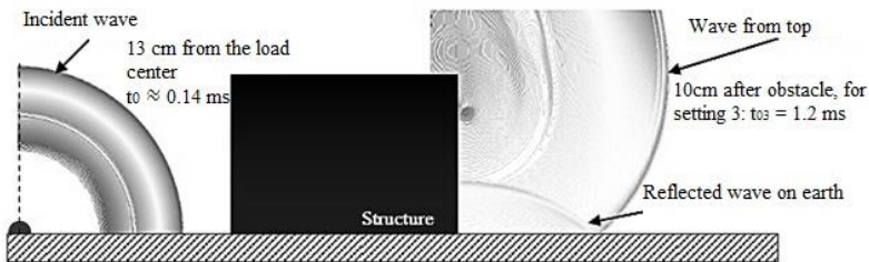
Fig. 6. Schematic representation of relaxation and reflection on the ground after configuration 3 obstacle
