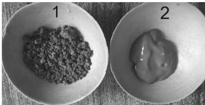
Fig. 3. General view of the components of the mixture: 1 - rigid loam; 2- drilling mud
