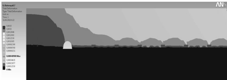
Fig. 5. Total deformations of rock mass in front of the stope face in the process of backfilling with the help of packs if height of the rocks being cut is 0.7 m
