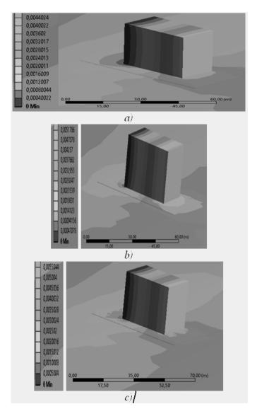
Fig. 8. Distribution of general deformation of soil foundation and nine-floor panel building at the face direction of the wave with  $P=10^7$  Pa, depending on the soil layering: *a* - loam 15 m - clay 5 m; *b* - clay 15 m - loam 5 m; *c* - sand 15 m - clay 5 m
