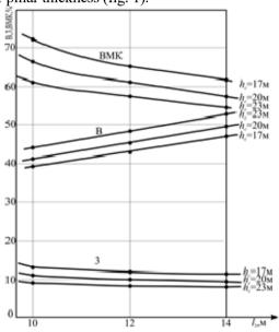
Fig. 1. Dependences graphs of losses *In*, a contamination Z and recovery of the BMK magnetite quartzites when developing by surface chamber system from thickness of a floor pillar of *hc* and distance between loading drives of  $l_3$
