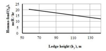
Figure 2 - the linear dependence of the gamma background  $\gamma_f$ on the height of the openings of the quarry  $h_y$
