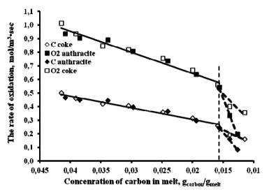
Fig. 15. The rate of oxidation of the carbon residue of coke and anthracite by carbon and oxygen. (air flow 18 l/h, T = 1250 K, fraction diameter 0.3 mm, melt height 65 mm, height of reagent injection 55 mm)
