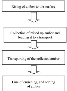
Fig. 6. Scheme of hydromechanical exception of amber
