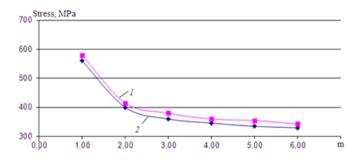
Fig.5. Dependence of stress on pipeline from depth of its laying at different diameters of pipeline: I - D=0,4 m, 2 - D=1,5 m
