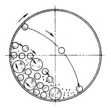
Fig. 2. Section of a reverse reaction chamber filled with a catalytic system consisting of a dispersing material (balls) and catalyst particles (points)
