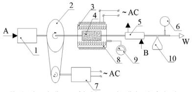
Fig. 1. Schematic diagram of the laboratory installation: 1 - feeder; 2 - transmission mechanism; 3 - the furnace; 4 - reactor; 6 - analytical control unit; 7 - the electric motor; 8 - heat insulation; 9 - thermocouple; 10 - condensate capacity. Flows: A - water (raw materials); W- gases of conversion
