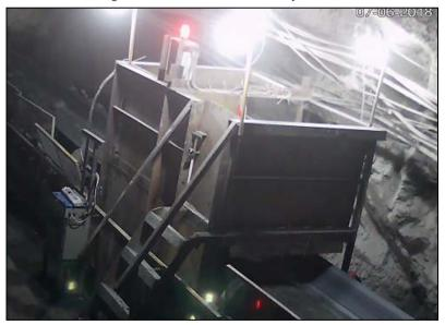
Fig. 7. - RCS on the conveyer in Nurkazgan underground mine
