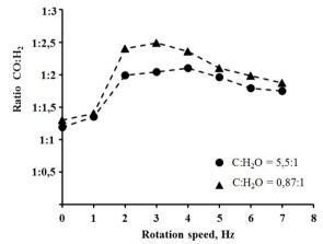
Fig. 9. Dependence of the change in the synthesis gas (CO:  $H_2$ ) ratio on the rotation speed
