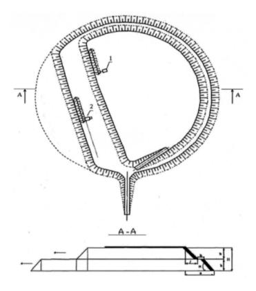
Fig. 2. Flow diagram of the selective formation of a double-deck external dozer dump: *1* - bulldozer; *2* - dump truck
