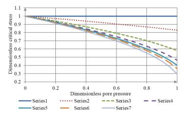
Fig. 4. Dependency of the relative breaking stress on the dimensionless pore pressure (according to the Hoek-Brown failure criterion)
