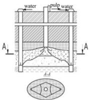
Fig. 2. Blurring of the next fall layer of productive horizon
