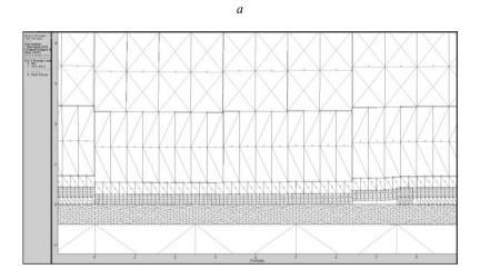
b Fig. 7. Model after longwall mining the bed on the length  $L_s$ = 20 m -*a* and  $L_s$ =80 m b
