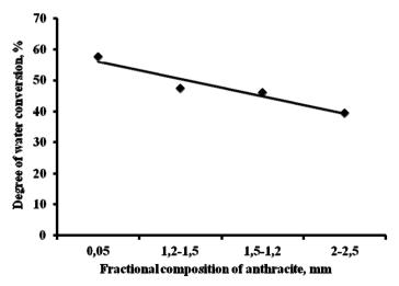
Fig. 13. Effect of the degree of water conversion from the fractional composition of anthracite (temperature 1233 K, initial concentration of coal 0,05 g carbon per g melt, water flow 0,1 g/min)
