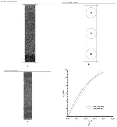
Fig. 5. Two-dimensional model of the *Strzelin* granite glued to the upper and lower grip a, location of the measurement circles on the sample b, displacement vectors c and stress-strain characteristics obtained after laboratory tests (—) and numerical simulations of uniaxial tension test (---)
