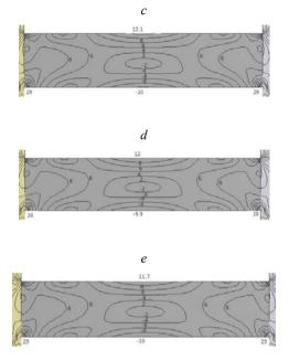
Fig. 2. Stress field development in 10 m crowns with the ore body dip of 90°, MPa; a-e – the crown of ores of 14-16, 13-15, 11-13, 10-11 and 9 points respectively
