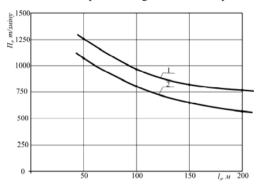
Fig. 3. Schedules of productivity dependence of load-haul-dumpers of  $\Pi_3$  from  $l_d$  ore delivery distance: 1 - TORO400E; 2 - EST-3,5
