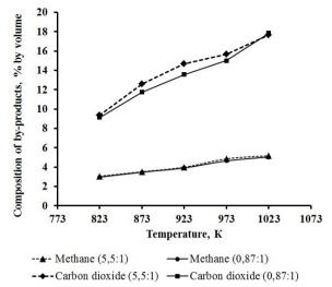
Fig. 5. Dependence of the yield of secondary products on temperature at different ratios of the initial reagent (C:H<sub>2</sub>O=0,87:1) and (C:H<sub>2</sub>O = 5,5:1)
