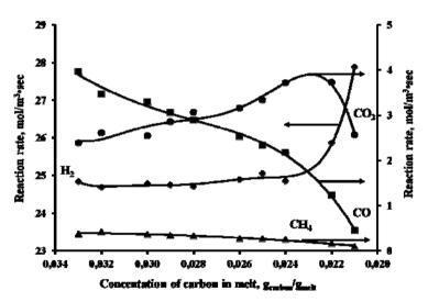
Fig. 14. Dependence of the reaction rate of the conversion of the carbon residue of anthracite (screen 2) with water on the concentration of carbon in the melt (water flow rate = 6,6 g/h, T=1270 K, coal fraction diameter 50  $\mu$ m, melt height 90 mm, reagent injection height 35 mm)
