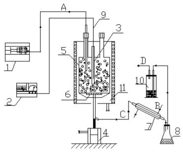
Fig. 10. Schematic diagram of a laboratory unit for processing hydrocarbons using AnCVB technology: 1 - syringe dispenser; 2 - control unit; 3 - thermocouple pocket; 4 - vibration control; 5 - reactor; 6 - metal-fiber filter; 7 - refrigerator; 8 - collection; 9 - thermocouple, 10 - bubbler; 11 - furnace.
