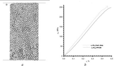
Fig. 4. The numerical model of the *Strzelin* granite sample before the simulation of the uniaxial compression test a and stress - strain characteristics obtained on the basis of laboratory uniaxial compression test (—) and numerical simulation (- - ) b
