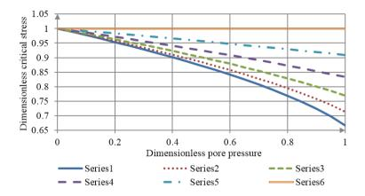
Fig. 7. Dependency of the relative breaking stress on the dimensionless pore pressure (according to the Shashenko failure criterion)
