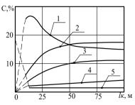
Fig. 1. Chart of the content change C: carbon (1), carbon monoxide (2), carbon dioxide (3), methane (4), carbon (5), along the length of  $l_k$  channel
