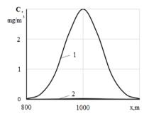
Figure 1 - Dependence of concentrations of CO (1) and  $NO_2(2)$ from the distance to the epicenter of the explosion
