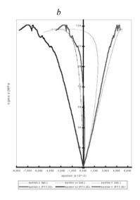
Because the subject of the research conducted by the author was the rocks behaviour in the field of tensile stresses, the next stage of the research were simulations of direct tensile tests using the PFC2D code.
