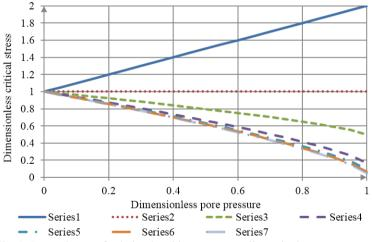
Fig. 1. Dependency of relative breaking stress on dimensionless pore pressure (according to the Bieniawski criterion)
