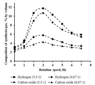
Fig. 7. Dependence of the yield of synthesis gas on the rotation speed for different ratios of the initial reagents (C:H<sub>2</sub>O=0,87:1) and (C:H<sub>2</sub>O=5,5:1)
