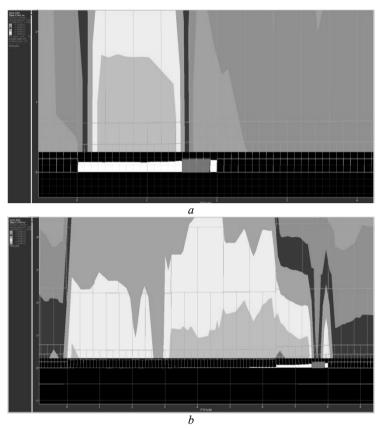
Fig. 9. Vertical stresses  $\sigma_z$  after the longwall minings of the bed were of  $L_s$ =20 m - a and  $L_s$ =80 m - b
