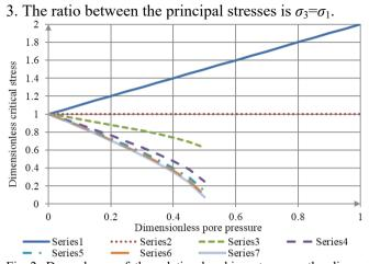
Fig. 2. Dependency of the relative breaking stress on the dimensionless pore pressure (according to the Bieniawski criterion)
