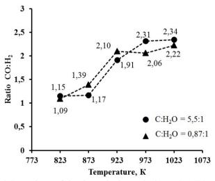
Fig. 6. Dependence of the change in the synthesis gas  $(CO:H_2)$  ratio on the conversion temperature
