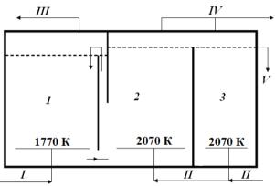
Fig. 11. Scheme of the reaction unit of technology in the melt for production of synthesis gas, *I-III* - three reaction zones of the reactor: *I* - conversion zone; *2* - oxidation zone; *3* - additional oxidation zone; *I* - Water, coal, CaCO<sub>3</sub>; *II* - Air; *III* - Synthesis gas; *IV* - Oxidation products; V - Slag
