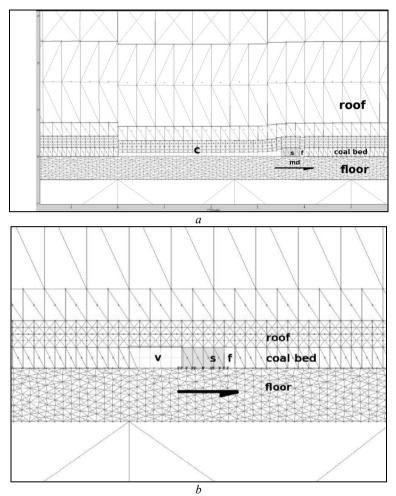
Fig. 6. Model with layers and deformable distinct elements zonation a and the immediate vicinity of a longwall face b; f – longwall face, s – mechanical hydraulic support; md – mining direction; c – cavity; v – void cavity
