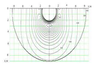
Fig. 2. Isobars of average hydrostatic pressure (in GPa) in plane rOz at different moments of time t=1,0 s
