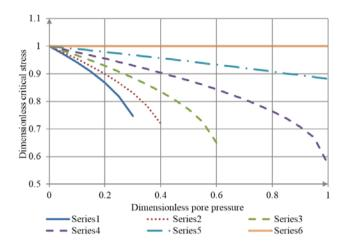
Fig. 9. Dependency of the relative breaking stress on the dimensionless pore pressure (according to the Shashenko failure criterion)
