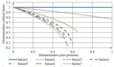
Fig. 5. Dependency of the relative breaking stress on the dimensionless pore pressure (according to the Hoek-Brown failure criterion)
