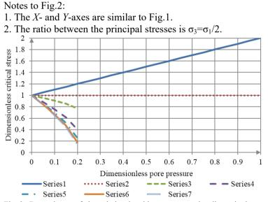
Fig. 3. Dependency of the relative breaking stress on the dimensionless pore pressure (according to the Bieniawski criterion)
