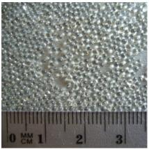
Fig. 3. General view of the dispersing material (glass beads)
