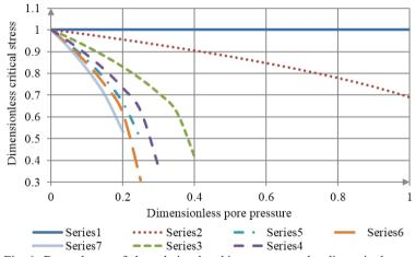
Fig. 6. Dependency of the relative breaking stress on the dimensionless pore pressure (according to the Hoek-Brown failure criterion)
