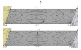
Fig. 3. Stress field development in 10 m crowns with the ore body dip of  $70^{\circ}$ , MPa; a-b – the crown of ores of 14-16 and 10-11 points respectively
