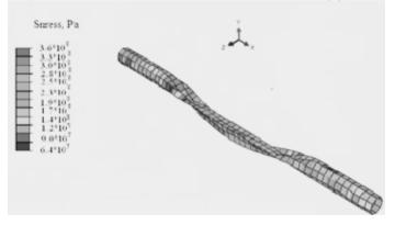
Fig. 4. Distribution of stresses in the steel pipe of 1.5 m in diameter at a laying depth of 5 m
