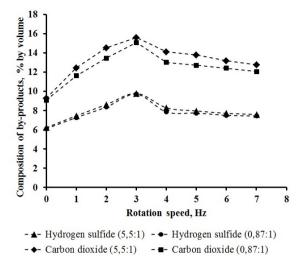
Fig. 8. Dependence of the yield of secondary products on the rotation speed for different ratios of the initial reagents (C:H<sub>2</sub>O=0,87:1) and (C:H<sub>2</sub>O=5.5:1)
