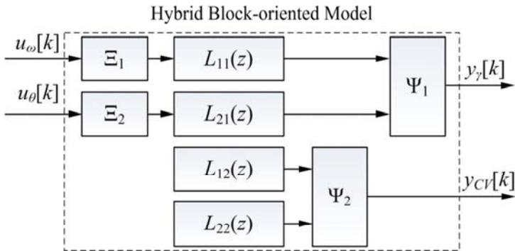
Fig. 5. Hybrid block-oriented model of ore crushing process
