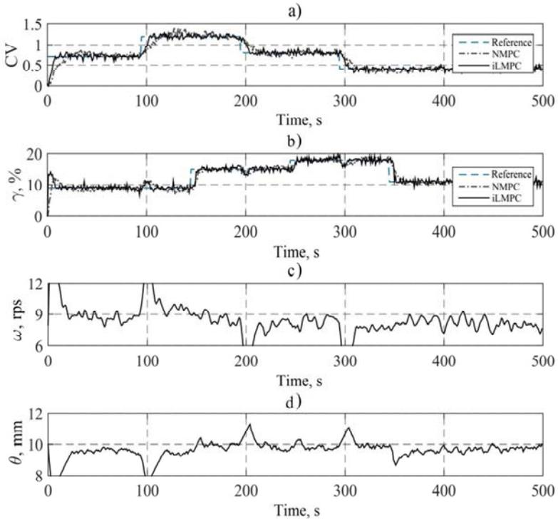
**Fig. 7.** Time series of the ore crushing process adaptive MPC control system with disturbances ( $\sigma_{CV} = 0,05$  and  $\sigma_{\gamma} = 0,5 \%$ )
