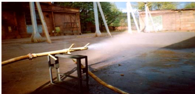
Fig. 8. Test cooling ejector "Dispersed" on the site of the mine to them. Lenin, PJSC "KRIVOJ ROG'S IRON-ORE COMBINE".
