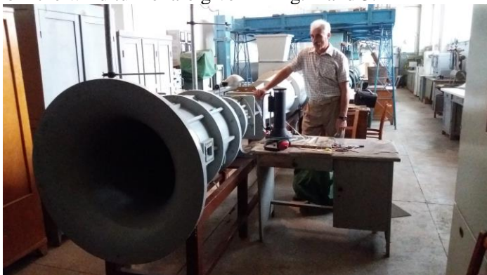
Fig. 2. The wind tunnel AT-2K-250/500 with the open flow and the closed test section
