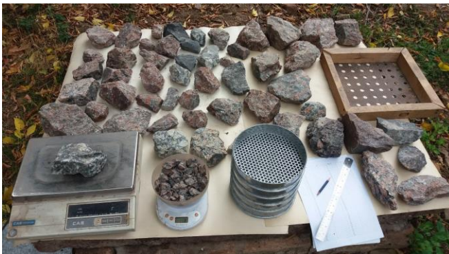
Fig. 1. The rock mass sample with size-sorted fractions
