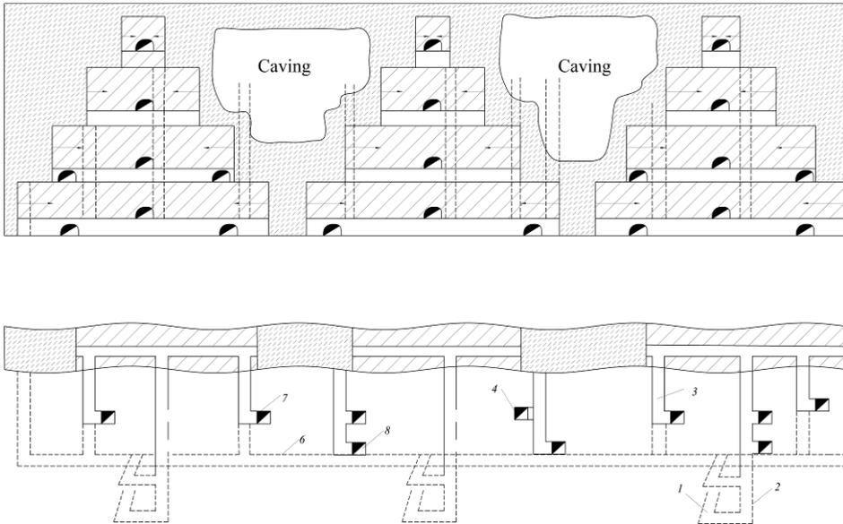
**Fig. 3.** Level development with three ramps: 1 – inclined drift; 2 – horizontal drift; 3 – haulage sublevel ort; 4 – ventilation-haulage ort; 5 – haulage crosscut of the main level; 6 – haulage drift of the main level; 7 – ore pass; 8 – raise.
