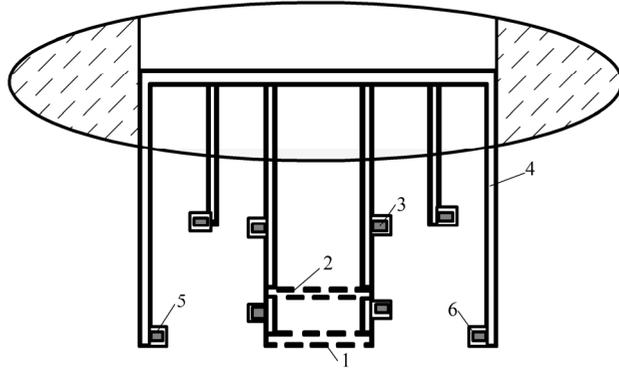
**Fig. 1.** Development mining of a level with an access ramp in the centre: 1 – inclined mine working of a ramp; 2 – horizontal mine working; 3 – haulage sublevel ort; 4 – ventilation-haulage ort; 5 – ore pass; 6 – raise.
